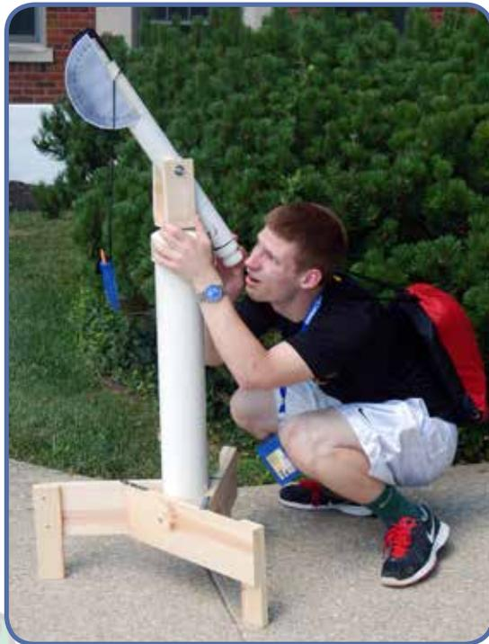
*The scholar-built telescopes prove to be useful tools not only for stargazing, but also for measuring heights and distances using the ancient triangulation method.*
